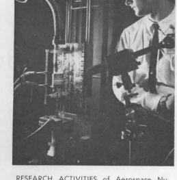
RESEARCH ACTIVITIES of Aerospace Nuclear Safety Department 7410 include special studies of reactor materials at high temperature. Frank Wessling (7411) uses an induction heater and vacuum system to investigate material interactions with graphite. Temperatures reach 5400 degrees F.
